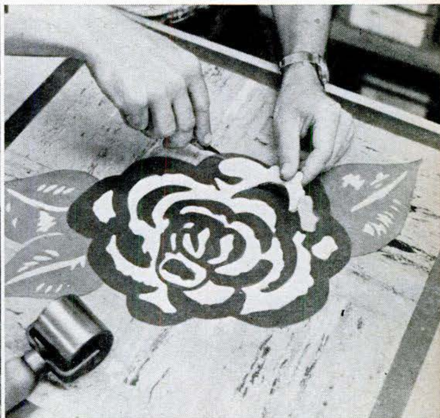
6 CUSTOM-MADE TILES carry out any design a customer wants. Here craftsman is forming a camellia of many cut-out parts that will fit like a jigsaw puzzle into molds cut into a four-tile background. Special lamp keeps tiles pliable as he works. END
